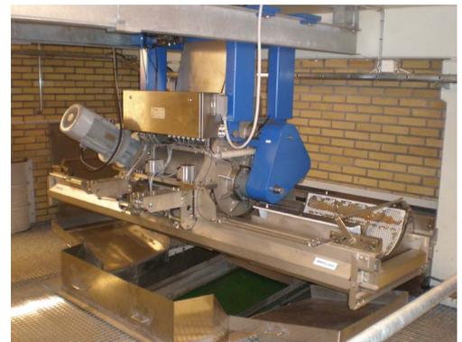
The Chopper with its grid exchange system
