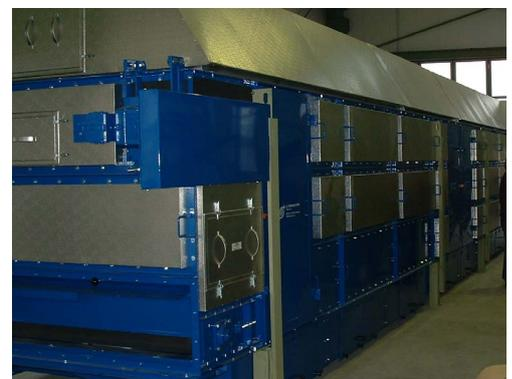
The belt dryer : direct drying stage
